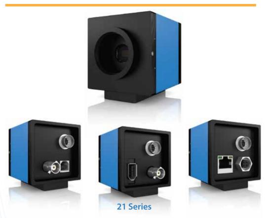
The Imaging Source "21" Series of CCD cameras are the perfect solution for many industrial automation, quality assurance, security, surveillance, and medical applications. Utilizing monochrome and color 1/4" Sony ICX098 sensors, this VGA format camera is available both in housed and board level versions with a choice of protocols including USB 2.0, Firewire 400, and Gigabit Ethernet.
