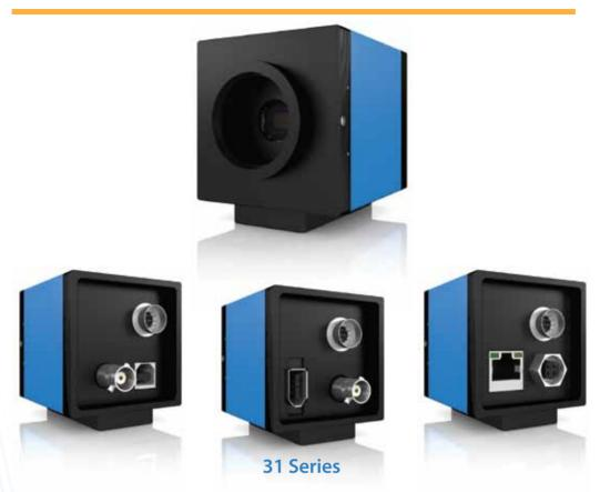
The Imaging Source "31" Series of CCD cameras are the perfect solution for many industrial automation, quality assurance, security, surveillance, and medical applications. Utilizing monochrome and color 1/3" Sony ICX204 sensors, this SVGA format camera is available both in housed and board level versions with a choice of protocols including USB 2.0, Firewire 400, and Gigabit Ethernet.
