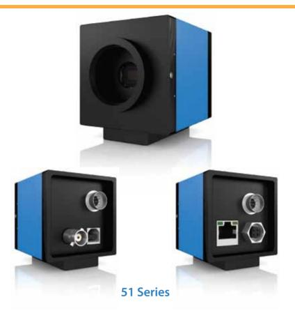
The Imaging Source "51" Series of CCD cameras are the perfect solution for many industrial automation, quality assurance, security, surveillance, and medical applications. Utilizing monochrome and color 1/2" Sony ICX274 Super HAD sensors, this 2 MegaPixel format camera is available with the choice of protocols including USB 2.0, and Gigabit Ethernet.
